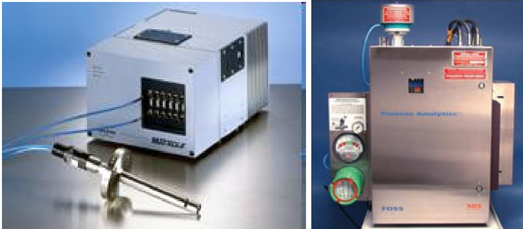
Figure 4. In situ near infrared spectrometer devices by Bruker (Matrix F FT-NIR) and by FOSS (XDS Process Analytics NIR).
