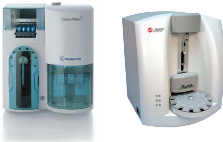
Figure 6. Automated at-line microscopes for analysis of cell number and viability with trypan blue staining; Cedex HiRes by Roche Innovatis and Vi-Cell by Beckman Coulter.
