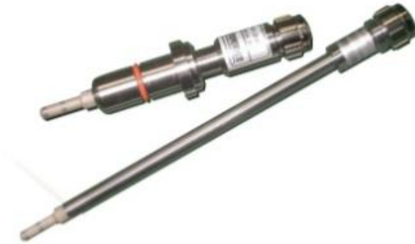
Figure 7. Aber cell density probe based on capacitance measurement.
